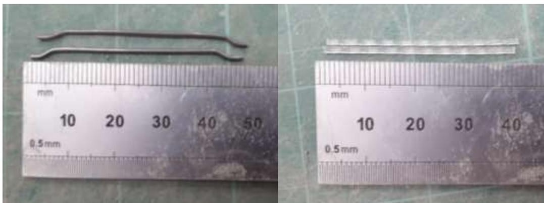
Figure 1: Individual Steel and Polypropylene Type 2 Synthetic Fibres
