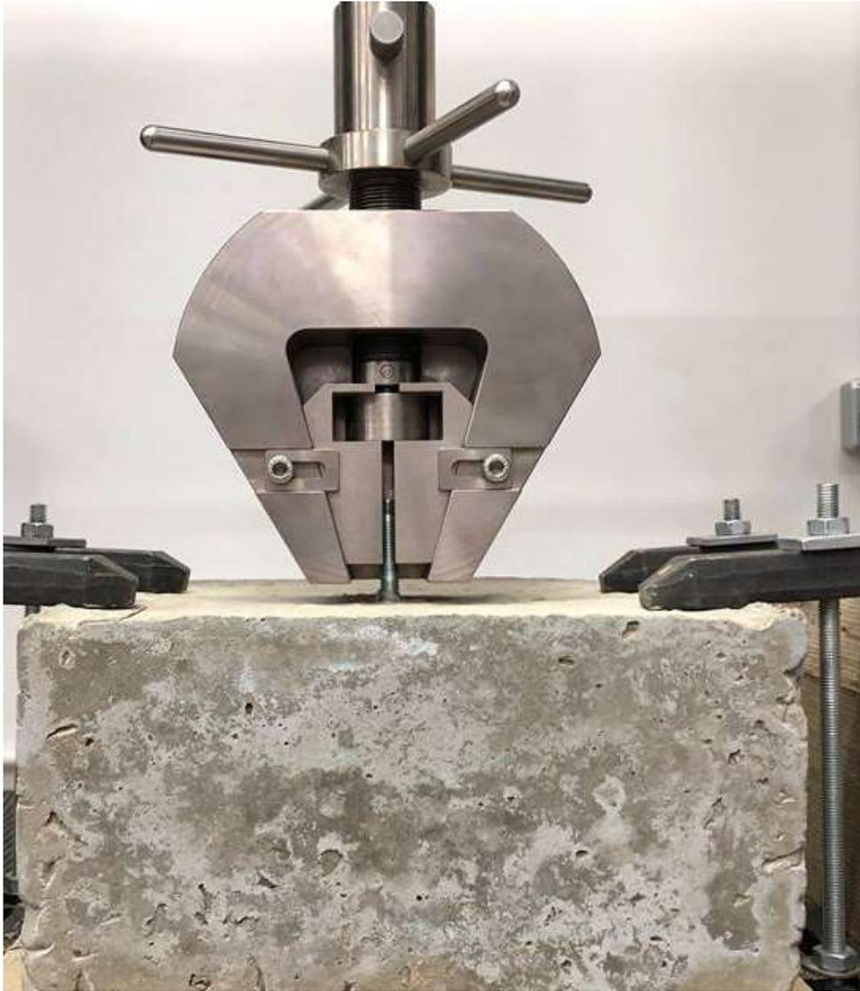
Figure 5 – Bolt pull out details, Lloyds LR100k apparatus
