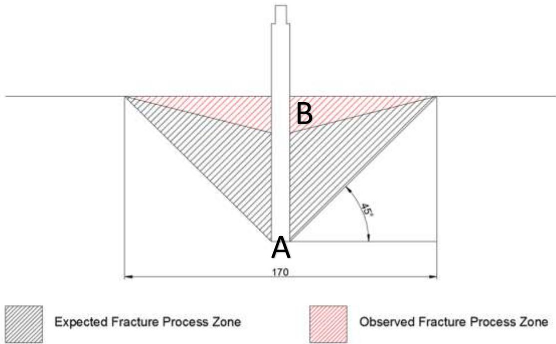
Figure 11 - Observed Fracture Zone
