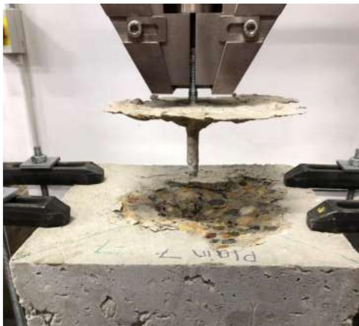
Figure 12: Cone failure of Slab 7
