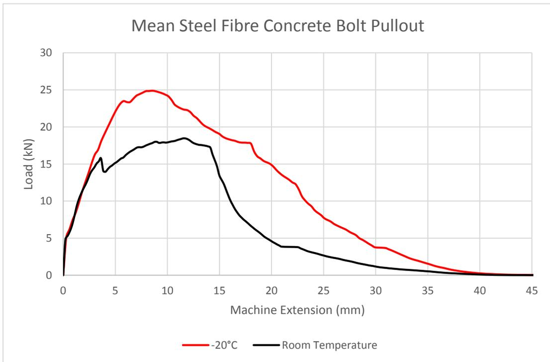
Figure 8 Steel Fibre Concrete Pull out Results
