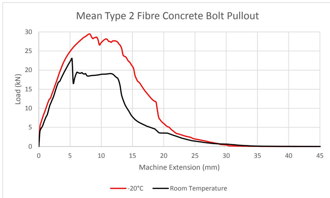
Figure 9: Polypropylene Fibre Concrete Pull out Results
