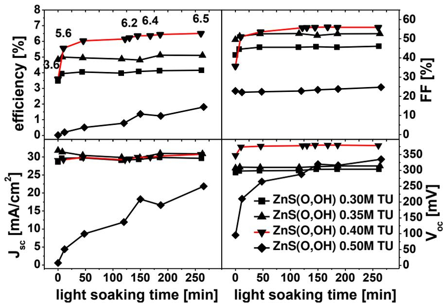
**Figure 6.** Evolution of device parameters with 1 sun light soaking time for devices with ZnS(O,OH) buffer layer deposited with different thiourea (TU) concentrations during the CBD process.
