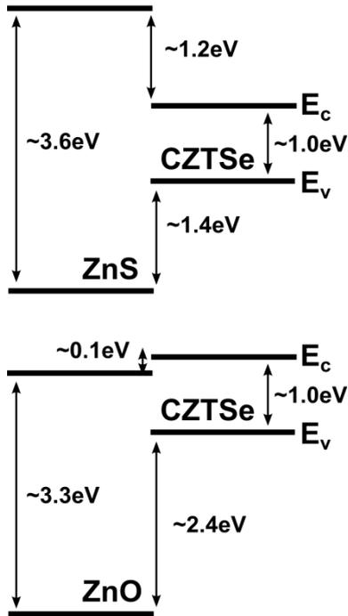
**Figure 2.** Approximation of band alignment of CZTSe absorber with ZnS (=” spike like”) and ZnO (=”cliff like”). Band offsets were taken from Barkhouse et al. <sup>[11]</sup> and adjusted to CZTSe absorber by shifting the valence band minimum according theoretical calculations. <sup>[17]</sup> A small spike like conduction band alignment ( $\Delta E_c < 0.5\text{eV}$ ) would be preferable, which could be achieved by tailoring the S/O ratio in Zn(O,S) <sup>[9]</sup>.
