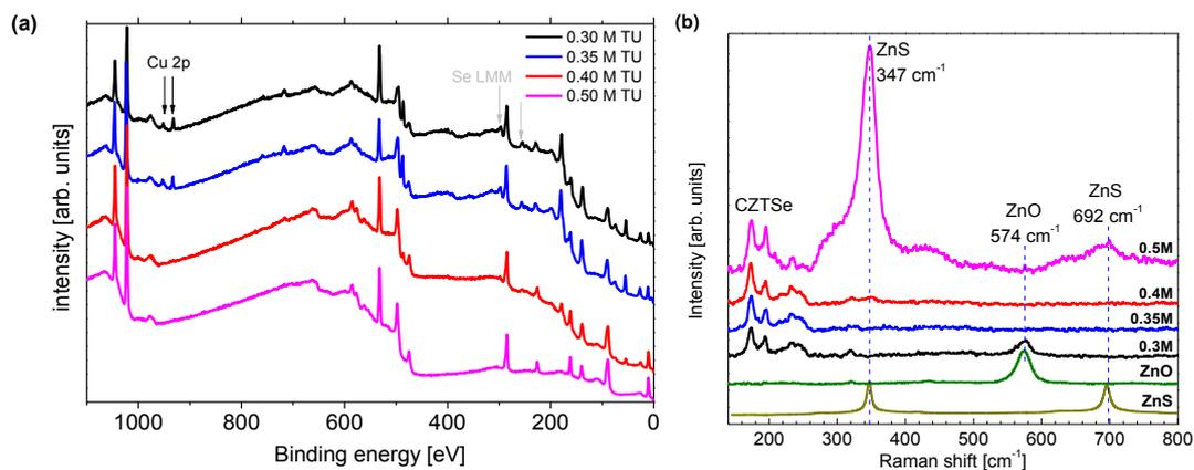
**Figure 8.** X-ray photoelectron spectroscopy (a) and UV-Raman (b) spectra and of ZnS(O,OH) buffer layer on CZTSe absorber deposited with different thiourea (TU) concentrations during the CBD process; ZnO and ZnS reference spectra were add for convenience.
