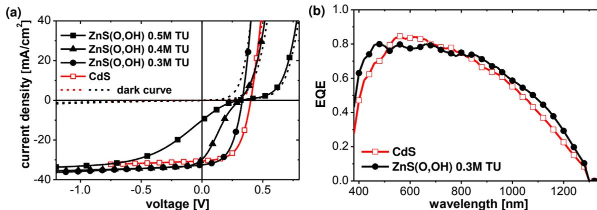
**Figure 3.** (a) Illuminated and dark JV curves of devices with ZnS(O,OH) buffer layer deposited with different thiourea (TU) concentrations during the CBD process and CdS as reference buffer layer. (b) External quantum efficiency of device with 0.3 M TU ZnS(O,OH) buffer and CdS buffer.
