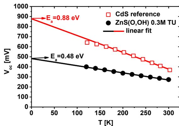
**Figure 4.** Temperature dependence of  $V_{oc}$  and linear extrapolation to  $T=0K$  to extract the activation energy of the recombination process for solar cells with ZnS(O,OH) 0.3 M TU and CdS buffer layers.
