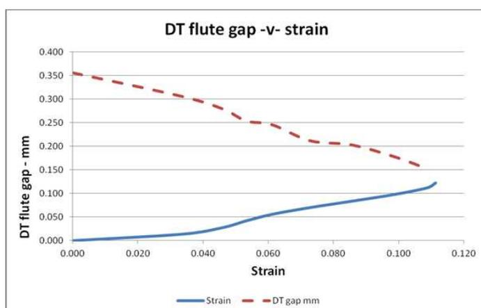
Figure 4 – DT Flute gap versus strain
