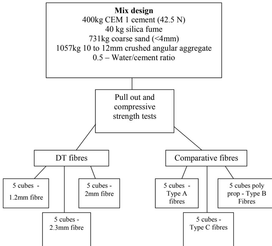
Figure 2 – Manufacturing chart/test program
