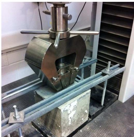
Figure 3. - Pull out testing arrangement of Lloyds testing apparatus
