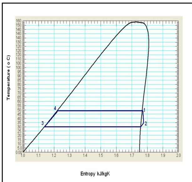
**Fig. 3** T-S diagram for the R-245fa cycle.
