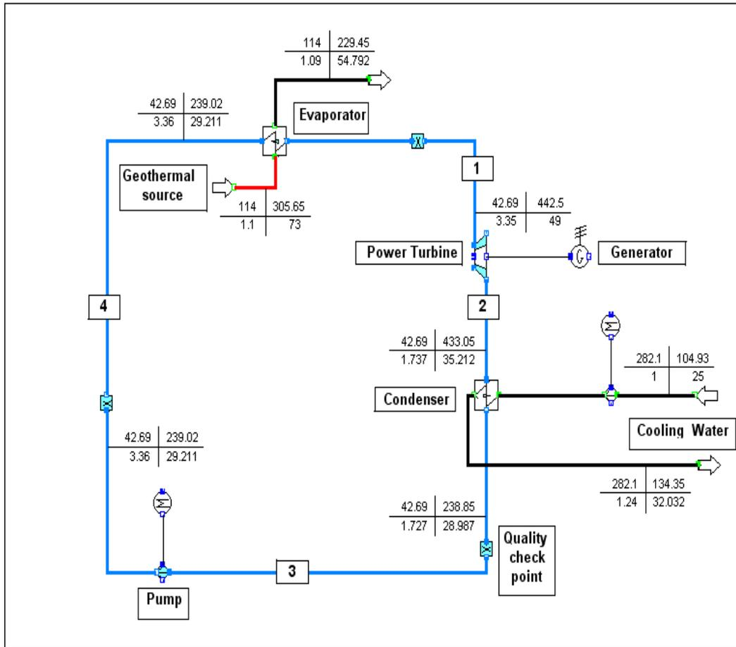
Fig. 4 Representation of the ORC cycle in IPSEpro.
