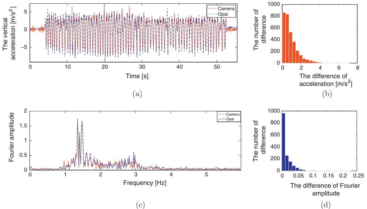
**Fig. 7.** (a) The comparison between the two accelerations of Subject 13 in T2 in the time domain. (b) The histogram of the displacement difference values between the camera and Opal. (c) The corresponding Fourier amplitude comparison with frequency from 0 to 6. (d) The histogram of the Fourier amplitude difference values between the camera and Opal.
