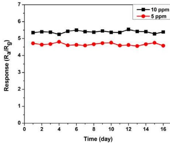
Fig. 11 long-term stability of the gas sensor based on  $\alpha$ -Fe<sub>2</sub>O<sub>3</sub> nanoparticles to 5 ppm and 10 ppm H<sub>2</sub>S gas at 300 °C
