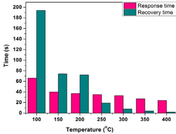
Fig. 7 Response time and recovery time of the sensor derived from  $\alpha$ -Fe<sub>2</sub>O<sub>3</sub> upon exposure to 10 ppm H<sub>2</sub>S gas at an operating temperature in the range of 100 °C- 400 °C.
