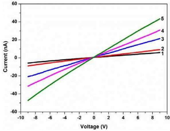
Fig. 5 I-V characteristics between the two neighboring electrodes bridged by the  $\alpha$ -Fe<sub>2</sub>O<sub>3</sub> film at different working temperature ranging from 100 °C to 350 °C
