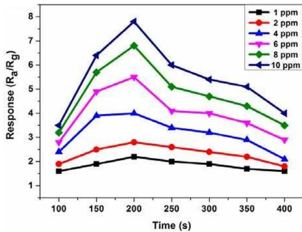
Fig. 6 (a) Gas response of the  $\alpha$ -Fe<sub>2</sub>O<sub>3</sub> based sensor to different concentrations of H<sub>2</sub>S gas measured at different working temperature.
