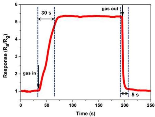
Fig. 8 Real-time gas sensing transients of the sensor based on  $\alpha$ -Fe<sub>2</sub>O<sub>3</sub> nanoparticles to 10 ppm H<sub>2</sub>S gas at 300 °C.
