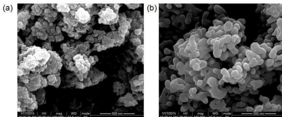
Fig. 3 SEM images of (a) the as-prepared  $\text{Fe}_3\text{O}_4$  precursor (b) the  $\alpha\text{-Fe}_2\text{O}_3$  product
