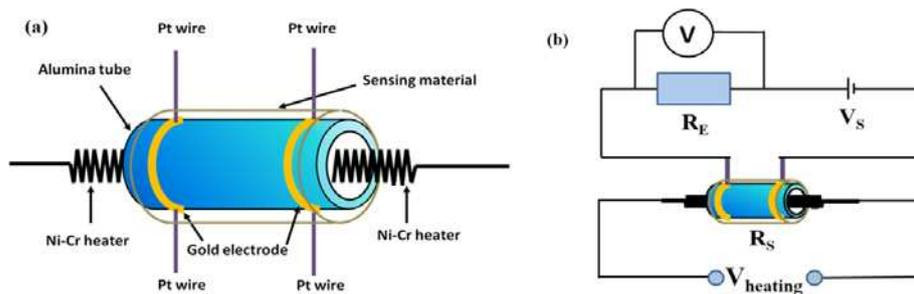
Fig.1 (a) Schematic of the gas sensor based on  $\alpha\text{-Fe}_2\text{O}_3$  nanoparticles. (b) The measuring electric circuit for the gas sensor
