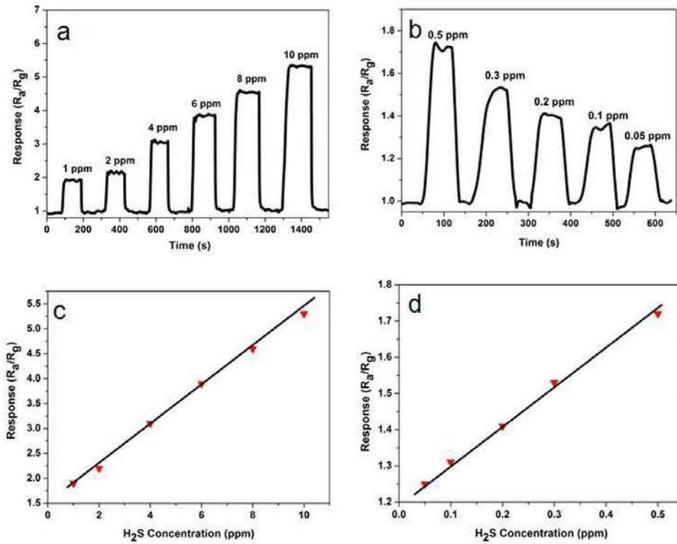
Fig. 9 Dynamic response-recovery curve of the  $\alpha\text{-Fe}_2\text{O}_3$  based sensor upon exposure to different concentration  $\text{H}_2\text{S}$  gas at the operating temperature of 300 °C: (a) 1 ppm -10 ppm, (b) 0.05 ppm-0.5ppm. Linear plot of sensitivity as a function of the concentrations of  $\text{H}_2\text{S}$  gas: (c) 1 ppm-10 ppm, (d) 0.05 ppm-0.5 ppm.
