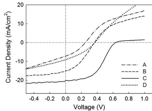
**Fig. 1.**  $J$ - $V$  curves of the best performing substrate devices obtained from each of the post-growth treatments A–D. See Table 2 and the text in Section 2 for a description of these treatments, and Table 3 for the associated solar cell performance parameters.
