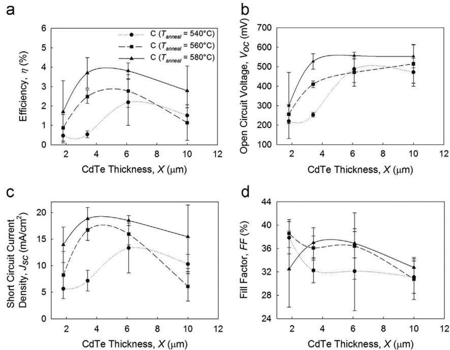
**Fig. 4.** Dependence of (a)  $\eta$ , (b)  $V_{OC}$ , (c)  $J_{SC}$  and (d)  $FF$  as a function of CdTe thickness for a range of annealing temperatures ( $T_{anneal}=540\text{--}580\text{ }^{\circ}\text{C}$ ). Lines added as a guide to the eye. The data points show the averages and standard deviation for up to 16 devices. See Table 4 for the best contacts from each plate.
