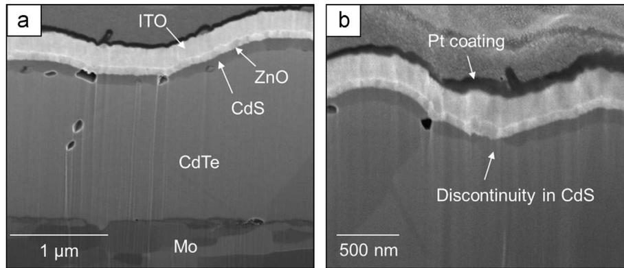
**Fig. 6.** Secondary electron images of FIB-milled ITO/ZnO/CdS/CdTe/Mo device cross-section: (a) Full device structure and (b) the junction region. The device was subject to treatment C, i.e. the double-anneal process, with  $T_{2nd}=580$  °C, and had efficiency,  $\eta=5.3\%$ .
