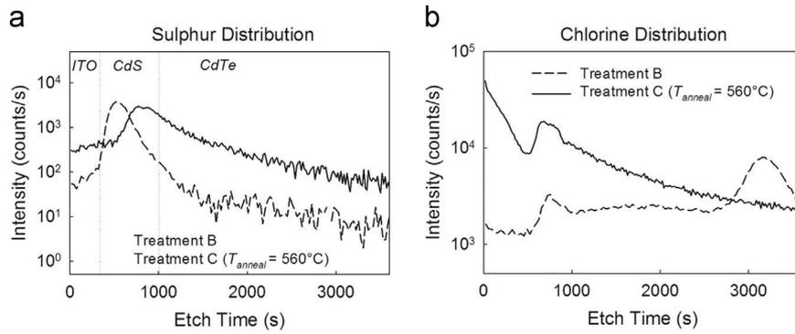
**Fig. 2.** SIMS depth-profiles of (a) sulphur and (b) chlorine concentrations in a device subject to treatment B (single-anneal) and a device subject to treatment C (double-anneal,  $T_{\text{anneal}}=560^{\circ}\text{C}$ ). The left edge of the plots represents the front surface of the cell, i.e. the ITO surface.
