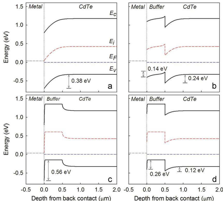
**Fig. 9.** Electronic band diagrams (at zero bias in the dark) generated using SCAPS focussing on the back contact region and the effect of the use of various buffer layers, each having a thickness of 500 nm. (a) No buffer layer, (b)  $N_A=10^{15} \text{ cm}^{-3}$  and  $E_{ea}=4.2 \text{ eV}$ , (c)  $N_A=10^{18} \text{ cm}^{-3}$  and  $E_{ea}=4.5 \text{ eV}$ , (d)  $N_A=10^{18} \text{ cm}^{-3}$  and  $E_{ea}=4.2 \text{ eV}$ .
