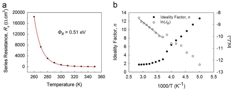
**Fig. 7.** (a) The temperature dependence of  $R_s$ , used to determine the back contact barrier height,  $\phi_B$ . (b) Temperature dependence of the ideality factor,  $n$ , and the saturation current,  $J_0$ . This data was taken from a device subject to treatment C ( $T_{anneal}=580$  °C), having a CdTe thickness of  $\sim 6$   $\mu\text{m}$  and for which  $\eta=5.5\%$ .
