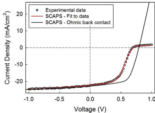
**Fig. 8.**  $J$ - $V$  data for highest efficiency ( $\eta=8.01\%$ ) substrate cell overlapped with modelled  $J$ - $V$  data from SCAPS software ( $\eta=8.02\%$ ). By inclusion of an Ohmic back contact in the model, the predicted performance was improved to 11.3%.
