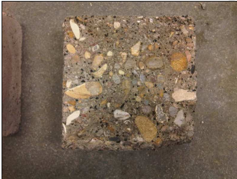
Figure 11 – Rubber particle distribution
