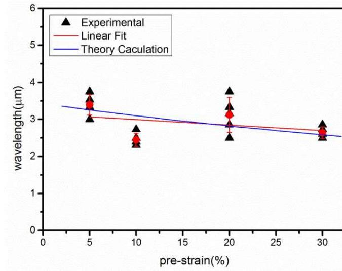
**Fig. 4.** The average wavelength of the wrinkles versus the applied pre-strain.
