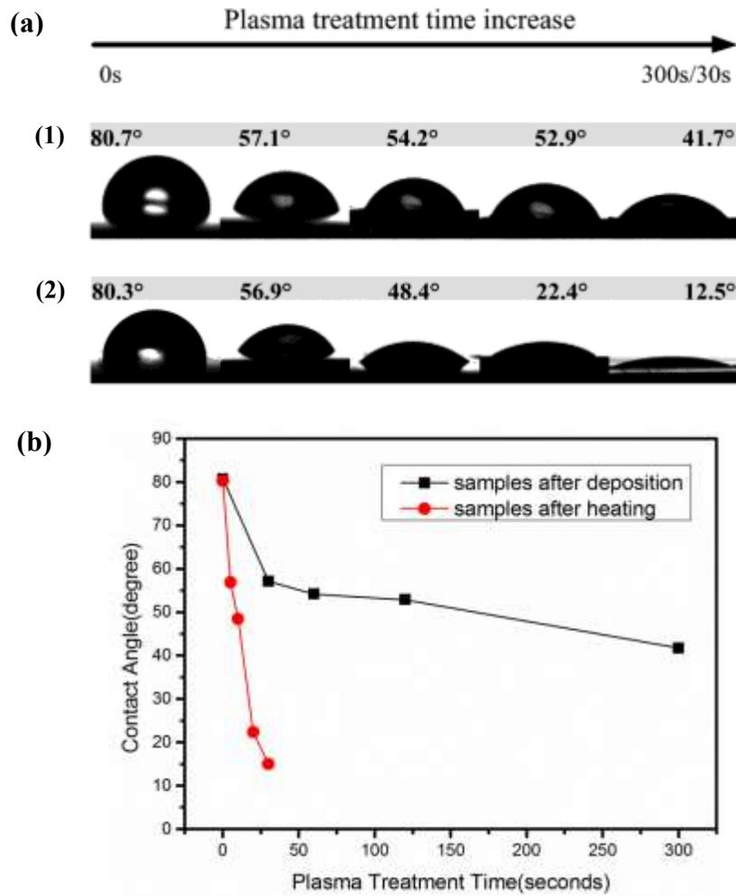
**Fig. 7.** (a) Snapshots for the water droplets on the surface of gold coated PS after (1) deposition; (2) post-annealing for different plasma treatment times. (b) Water contact angles versus plasma treatment time.
