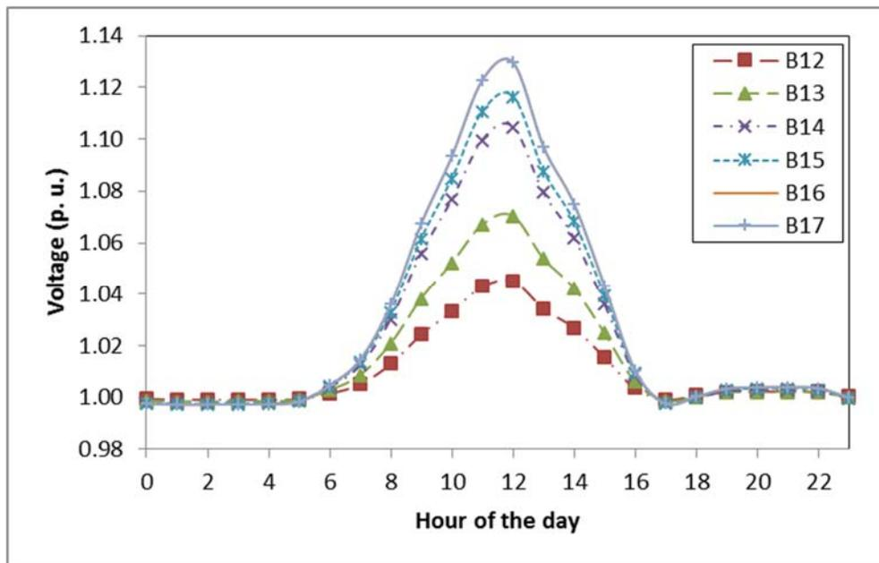
Fig. 8 Voltage profile along the 400 V feeder for an average Wednesday in May for PV penetration scenario S(100,100)<sup>1</sup>
