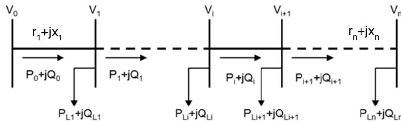
Fig 4 Representative diagram of radial distribution network parameters
