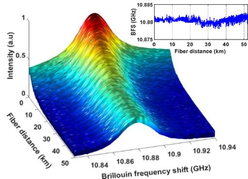
Fig. 11. Brillouin gain spectrum over sensing fiber distance
