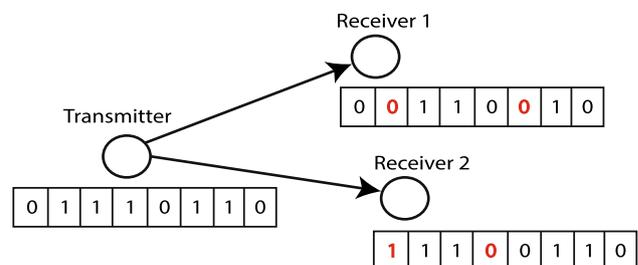
**Fig. 2** Illustrating binary symmetric broadcast channel. A binary vector broadcast by the transmitter is overheard by two stations. Reception may be lossy, with bits being received flipped at receiver  $i$  with probability  $p_i$  (example bit flips are indicated in red bold) (Color figure online)
