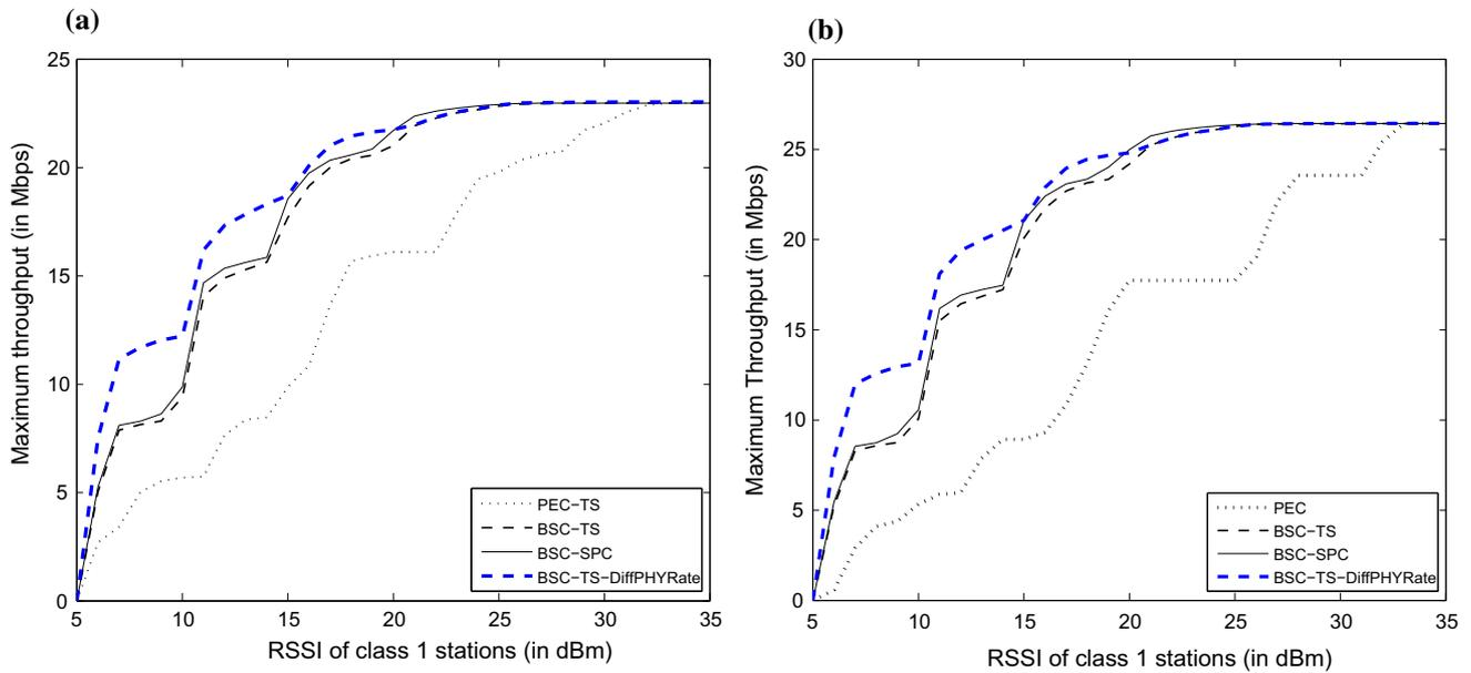
**Fig. 7** Multicast per-station maximum throughput versus RSSI of class 1 stations,  $L = 8000$  bytes,  $n_1 = n_2 = 10$  stations. TS and SPC indicate time-sharing coding and superposition coding respectively. **a**  $L = 8000$  bytes. **b**  $L = 65,536$  byte
