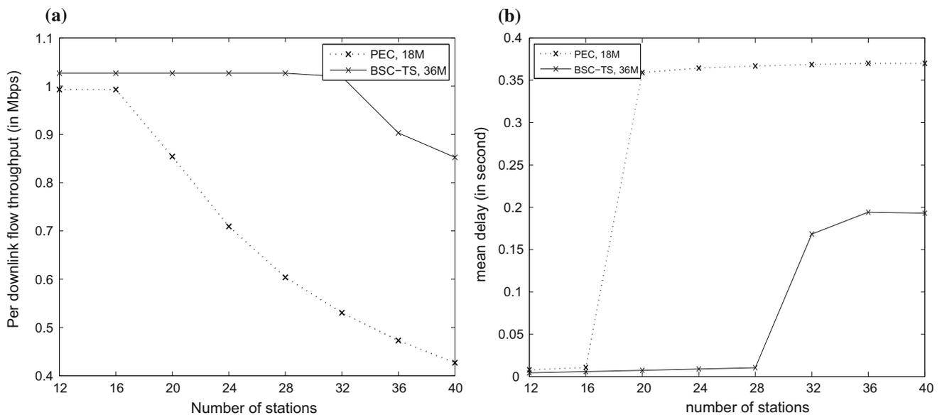
**Fig. 10** Per downlink flow throughput and mean downlink delay vs number of stations, outdoor measurement channel data, RSSI of class 1 18 dBm, RSSI of class 2 33 dBm. **a** Per downlink flow throughput. **b** Mean downlink delay
