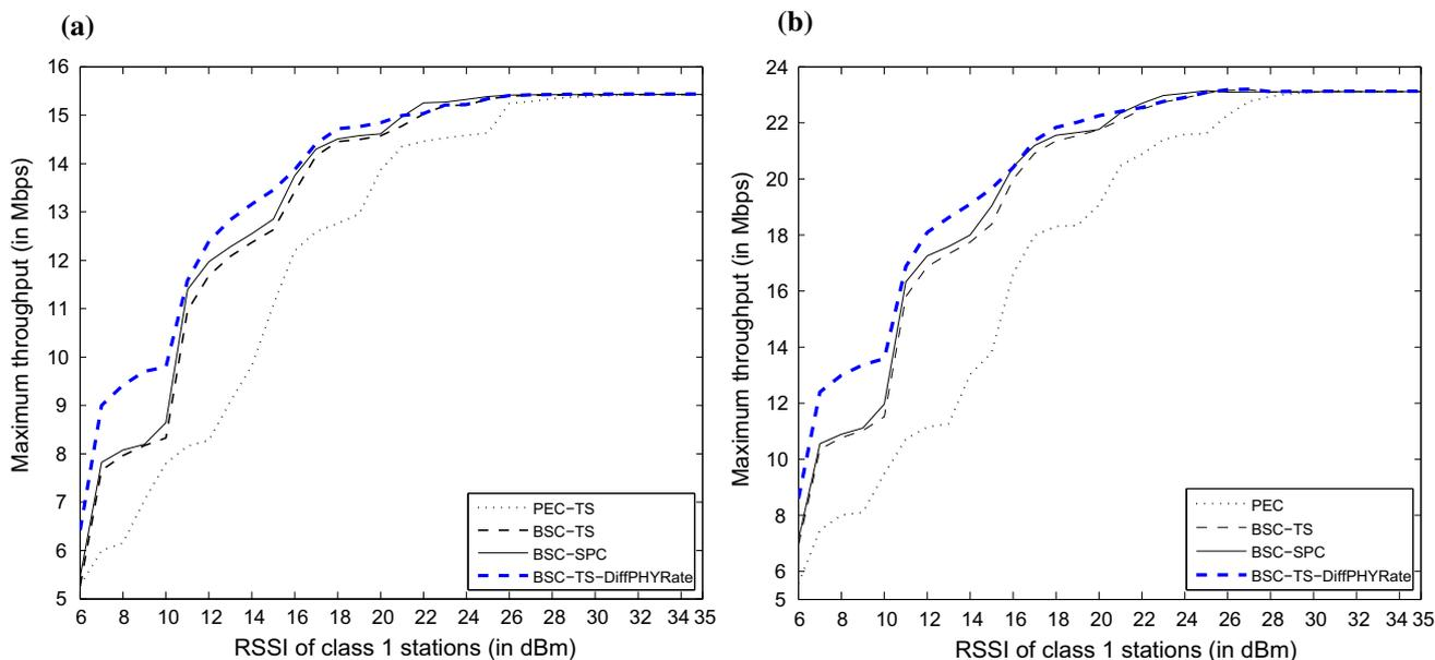
**Fig. 5** Unicast maximum network throughput versus RSSI of class 1 stations,  $L = 8000$  bytes. TS and SPC indicate time-sharing coding and superposition coding respectively. **a**  $n_1 = n_2 = 10$  stations. **b**  $n_1 = n_2 = 5$  stations
