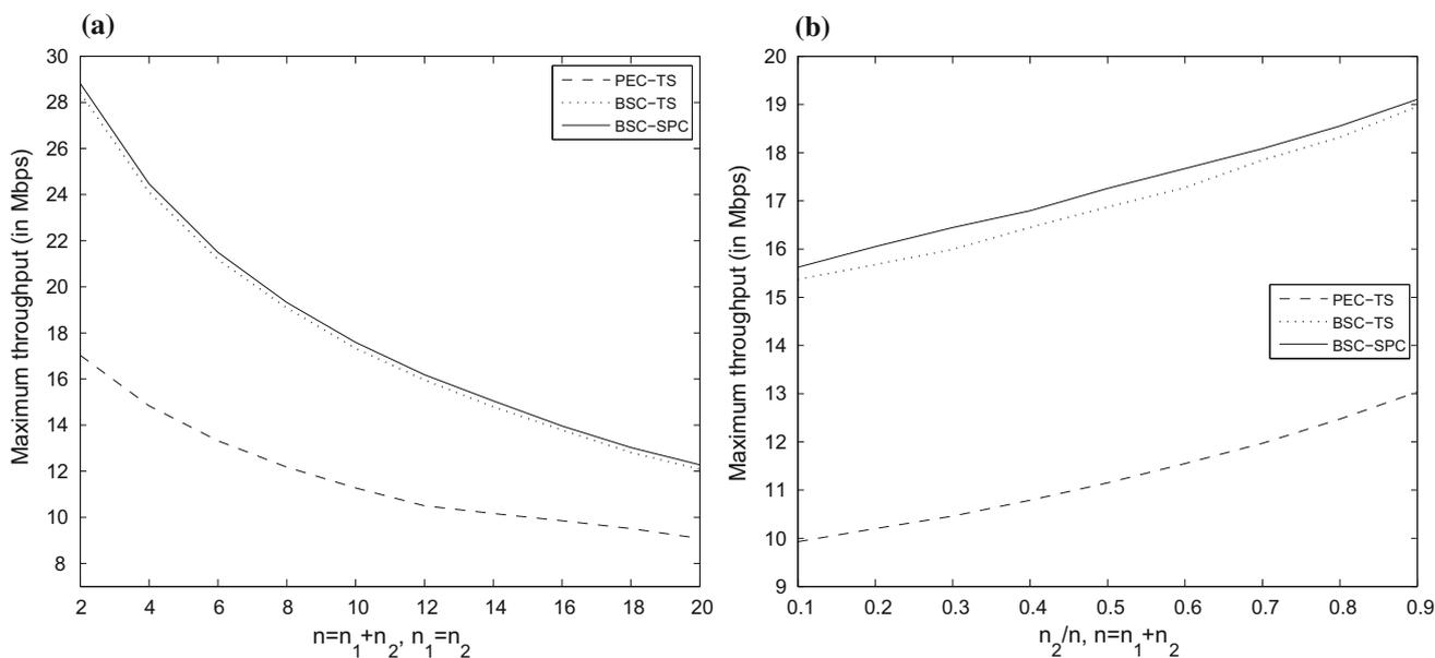
**Fig. 6** Unicast maximum network throughput,  $L = 8000$  bytes. TS and SPC indicate time-sharing coding and superposition coding respectively. **a**  $n_1 = n_2, RSSI = 13$  dBm. **b**  $n_1 + n_2 = 10, RSSI = 12$  dBm
