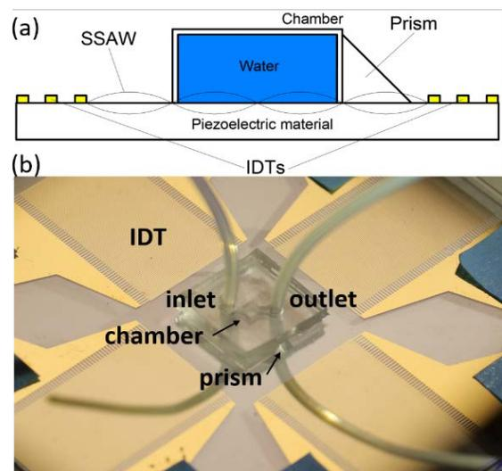
FIG. 1. (a) Schematic of surface acoustic wave (SAW)-based device. (b) Optical image of device after fabrication, showing interdigital transducers (IDTs), polydimethylsiloxane (PDMS) chamber, prism, inlet, and outlet.
