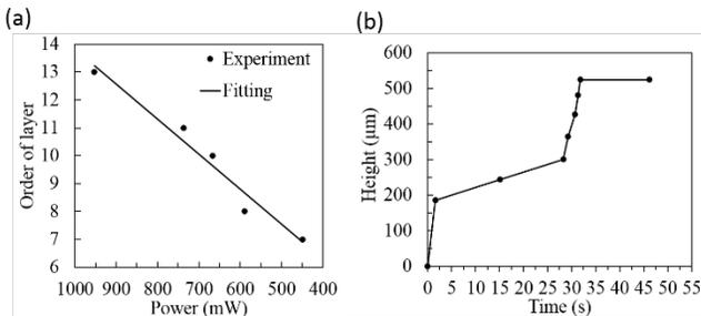
FIG. 5. (a) Changes of layer order of 10- $\mu\text{m}$  microparticles when input power was decreased (side view of X axis). (b) Levitation height of 10- $\mu\text{m}$  microparticles from bottom layer with time for an input power of 4,380 mW.
