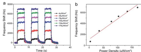
Fig. 6 (a) Photo responses of the SAW photodetector based on  $\text{Bi}_2\text{S}_3$  nanobelts under 625 nm visible light with different power densities. (b) The dependence of frequency shift on power intensities under 625 nm visible light.
