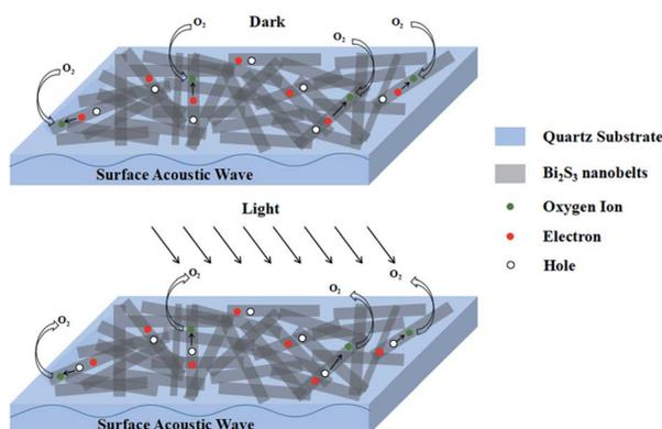
Fig. 7 Schematic illustration of sensing mechanisms of adsorption and desorption of oxygen on Bi<sub>2</sub>S<sub>3</sub> nanobelts.
