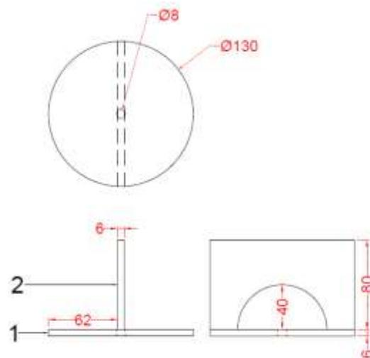
**Figure 6.** Top fixture for applying tension/compression loading
