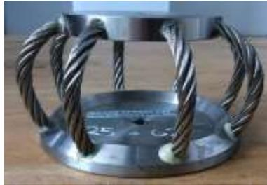
**Figure 1.** Polycal Wire Rope Isolator (PWRI)
