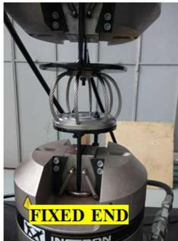
**Figure 4.** Loading Test of WRI in Vertical Directions
